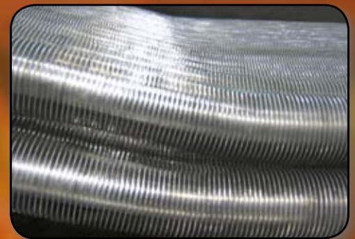
Tube bending that absorbs thermal expansion
